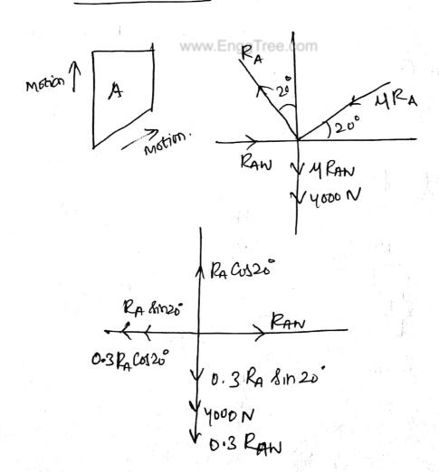
EnggTree.com Using eignilebrium, Shy 50, RA ast 20 - 4000 - 0.3 RAW - 0.3 RA 8m20 = 0 SFx =0, RAW - RA KM 20 - 0-3 RA CUS 20° =0 RAW = 0.34 PA + 0.281 RA RAW = 0.621 RA -(D) Sub in O 0.98 RA -4000 - 0.3 (0.621 RA) - 0.102 RA =0 0.641 RA =4000 www.Engglac. 5 b 233 N. RAW = 0.621 (6233) PAN = 3870 N 0.3 RRF 1 RBF (0.3RA 81720
