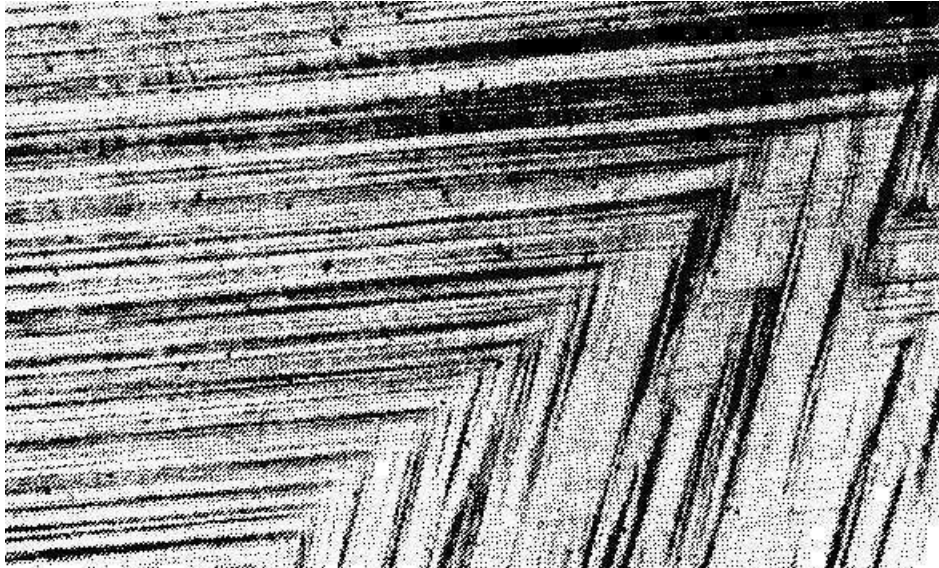
Figure 5.3 Slip lines in copper.
