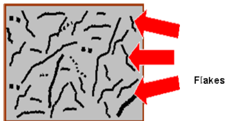
Figure 1.5 Graphite Flakes in Gray Cast iron
