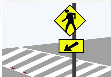
Figure: In-Pavement Raised Markers with Amber LED Strobe Lighting and LED Signs
