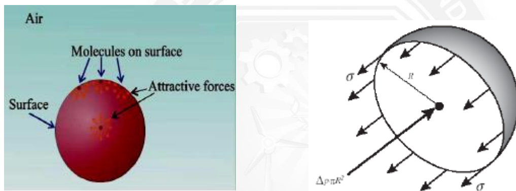
Figure 1.3.3 Surface Tension inside a Water Droplet
