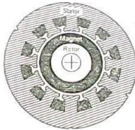
Figure 2.1.1 construction of BLPMDC motor
