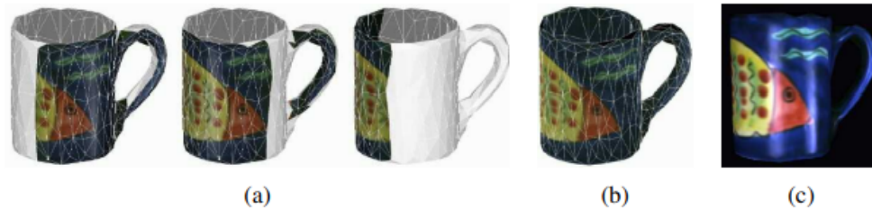
Figure 13.31 Estimating the diffuse albedo and reflectance parameters for a scanned 3D model (Sato, Wheeler, and Ikeuchi 1997) © 1997 ACM: (a) set of input images projected onto the model; (b) the complete diffuse reflection (albedo) model; (c) rendering from the reflectance model including the specular component.
