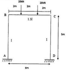
14. (a) Determine the support reactions on the frame by flexibility method.
