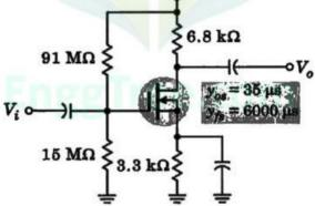
Find the output voltage  $V_0$ , for the input voltage  $V_{in} = 4$  mV.
